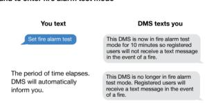
If you wish to stop being in fire alarm test mode at any time, follow the command below.
